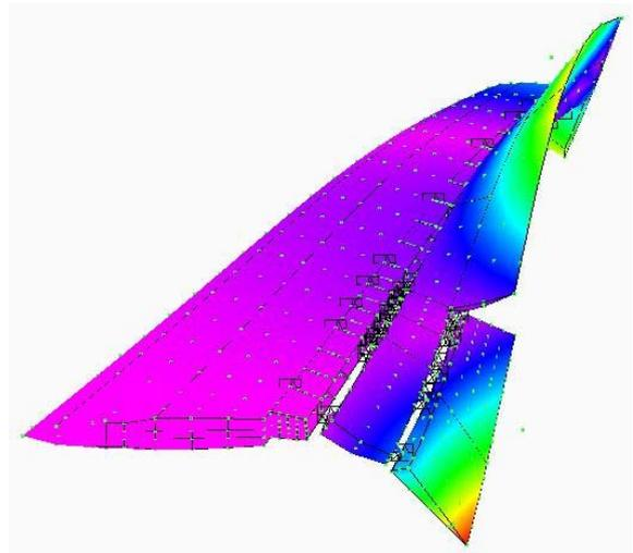
**Figure 15: Free Vibration Mode Shape of the nominal structure; Frequency = 18.24Hz**
