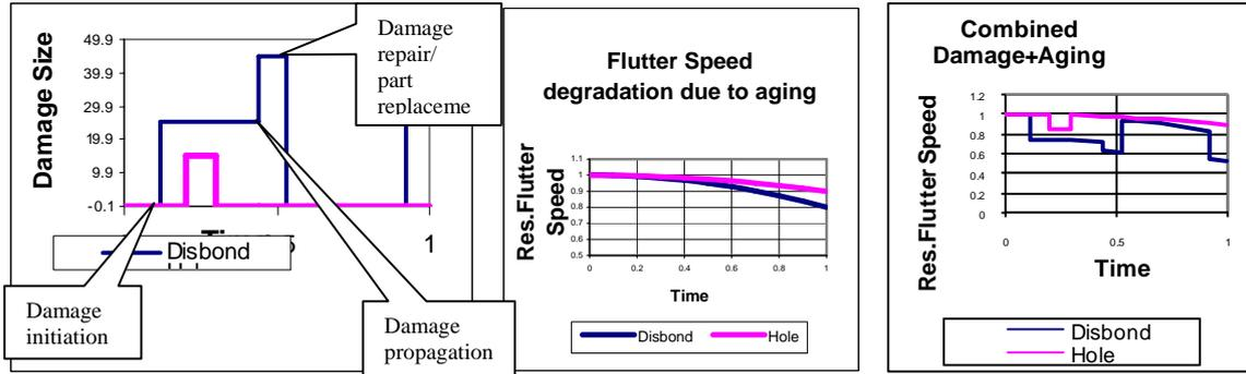
**Figure 1: Simulated Histories of residual flutter speed variation with time, as affected by damage, aging, and repair**
