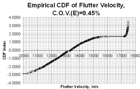
**Figure 16: CDF for Vertical Tail Flutter Velocity**
