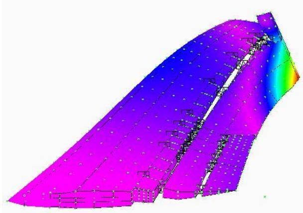
**Figure 14: Free Vibration Mode Shape of the nominal structure, Frequency = 16.34Hz**
