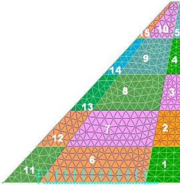
**Figure 2: Simple Wing Panels and Mesh**
