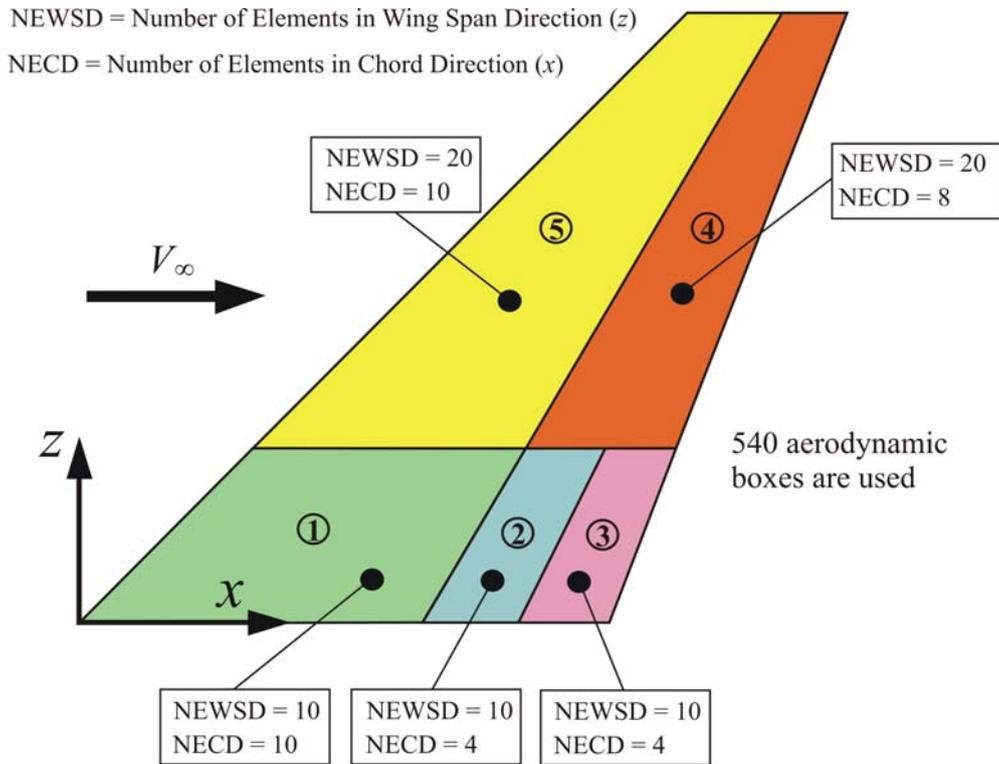
**Figure 13: Vertical Tail: Aerodynamic Model (Doublet Lattice Method)**
