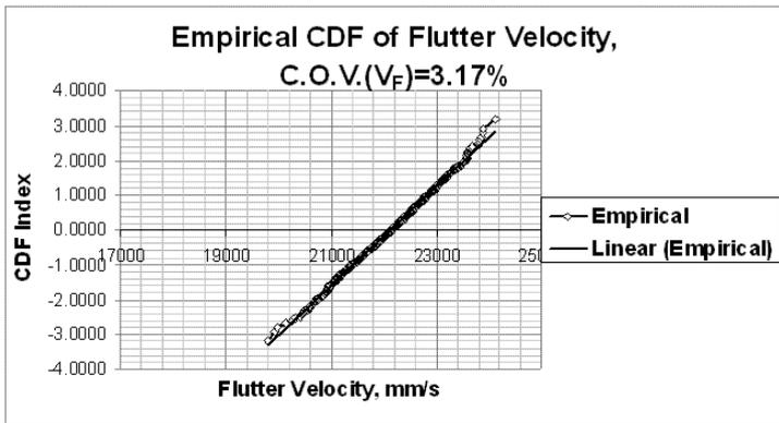
Figure 3: CDF of Flutter Speed in Normal CDF scale.
