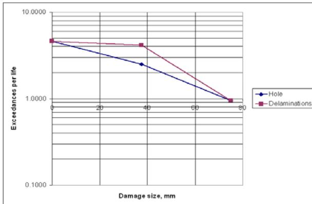
**Figure 19: Damage Exceedance Curve**
