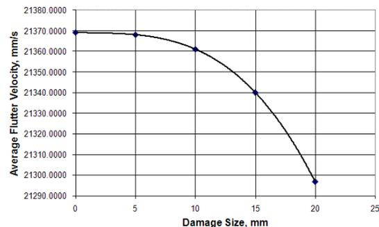
Figure 11: Average Flutter Velocity vs. Expected Damage
