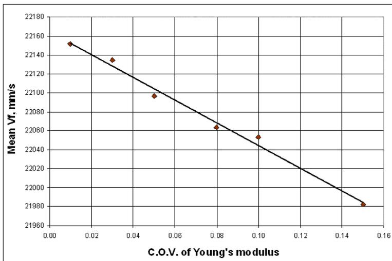
**Figure 7. Mean Flutter Velocity vs. C.O.V. of E**
