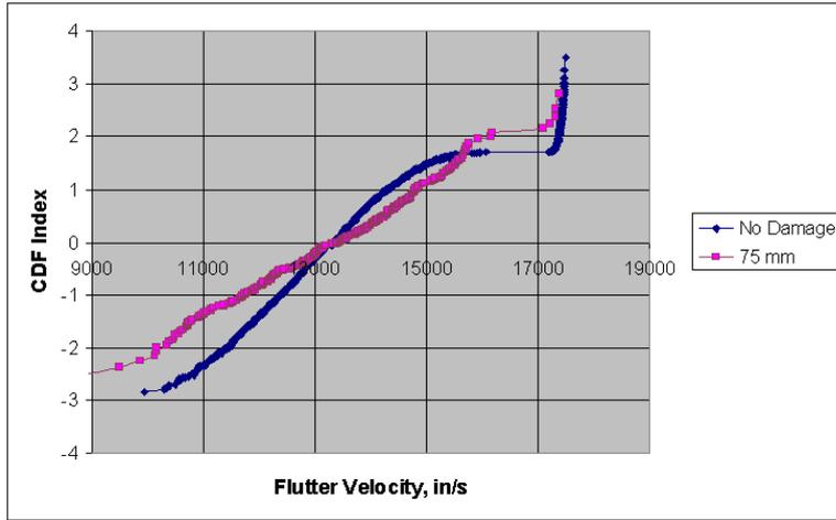
**Figure 18: Empirical CDF of  $V_F$  for damaged and undamaged structure**
