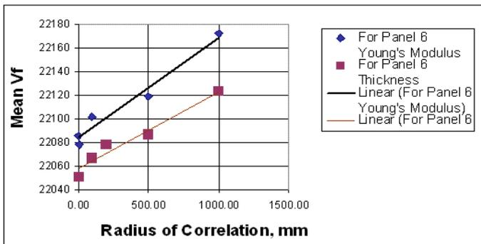
Figure 9: Average Flutter Velocity vs. Radius of Correlation
