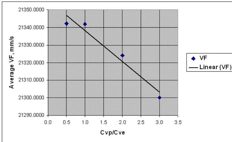
Figure 8: Effect of Cvp/Cve ratio on  $V_F$
