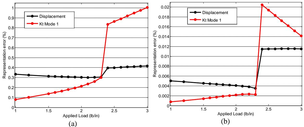
**Figure 8. Representation errors  $\varepsilon_{rep}$  of the displacements under uniform load and of the first eigenvector of the corresponding tangent stiffness matrix. Clamped-clamped curved beam (a) ROM 4L4D (b) ROM 6L7D.**
