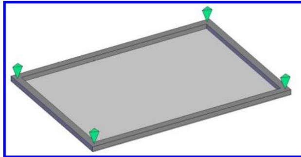
**Figure 3. Beam stiffened plate supported at its four corners.**
