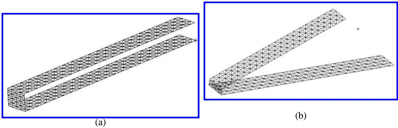
Figure 10. Finite element models of the PrandtlPlane configurations considered.
