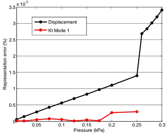
**Figure 15. Representation error  $\varepsilon_{rep}$  of the displacements under downward uniform load on the top wing and of the first eigenvector of the corresponding tangent stiffness matrix, unswept wing, 22-mode model.**
