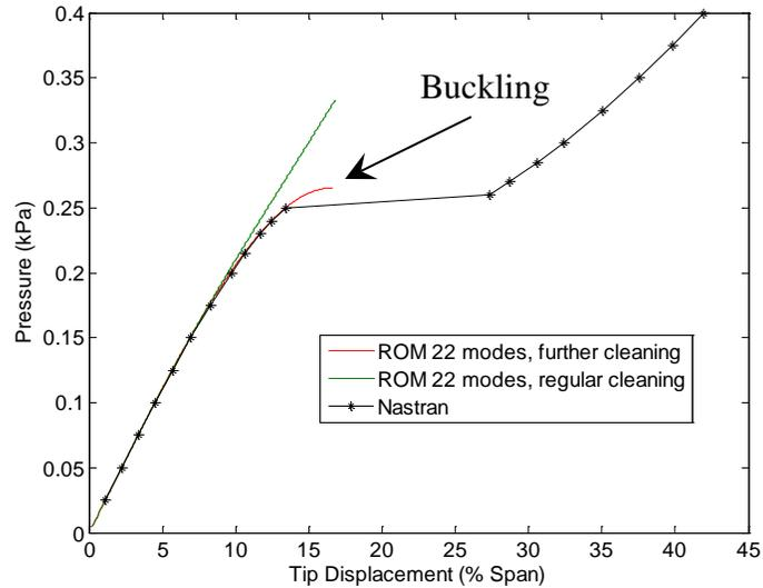
**Figure 18. Tip displacement of unswept wing vs. downward uniform pressure on upper wing only. Nastran and ROM predictions.**
