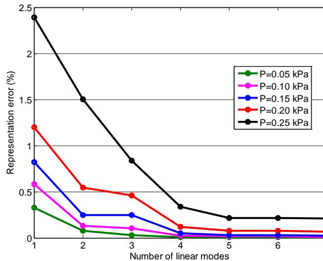
Figure 12. Representation error of the unswept wing, Fig. 10(a), as a function of the number of linear modes for various downward uniform pressures on upper wing only.
