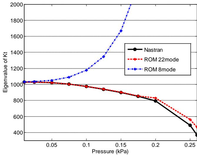
**Figure 14. Lowest eigenvalue of the full Nastran unswept wing model tangent stiffness matrix, of its projection on the 8-mode and 22-mode bases as functions of the magnitude of the downward uniform applied load.**
