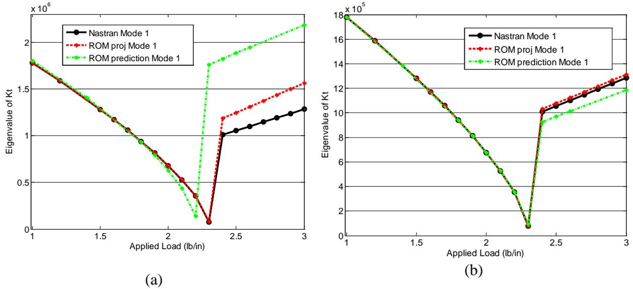
**Figure 9. Lowest eigenvalue of the full Nastran clamped-clamped curved beam model tangent stiffness matrix, of its projection on the ROM basis, and of the ROM, all as functions of the magnitude of the uniform applied load. (a) ROM 4L4D (b) ROM 6L7D**
