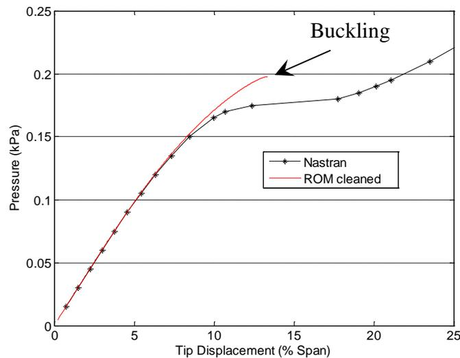
**Figure 19. Tip displacement of swept wing vs. downward uniform pressure on upper wing only. Nastran and ROM predictions.**
