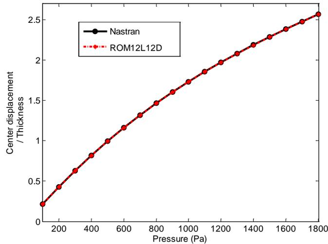
**Figure 5. Transverse displacement of the beam stiffened plate center predicted by both the reduced order model and the full finite element model.**
