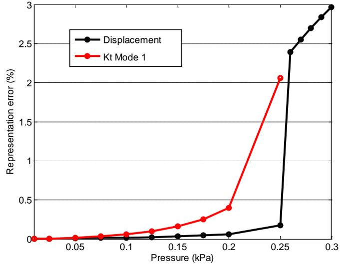
**Figure 13. Representation error  $\varepsilon_{rep}$  of the displacements under downward uniform load on the top wing and of the first eigenvector of the corresponding tangent stiffness matrix, unswept wing, 8-mode model.**
