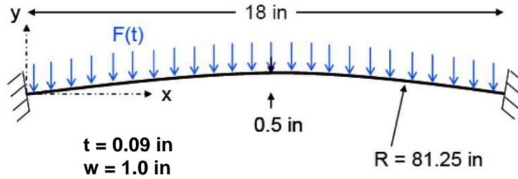
**Figure 6. Clamped-clamped curved beam geometry.**
