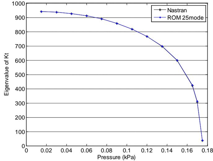
**Figure 17. Lowest eigenvalue of the full Nastran swept wing model tangent stiffness matrix and of its projection on the 25-mode bases as functions of the magnitude of the downward uniform applied load.**
