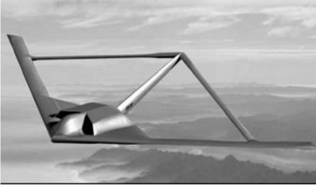
**Figure 1. Boeing Sensor-Craft Concept.**
