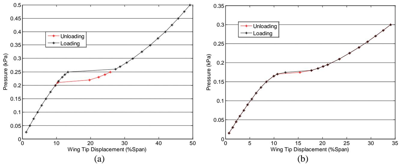
Figure 11. Load- wing tip displacement behavior. Wings of Fig. 10 with downward uniform pressure on upper wing only.
