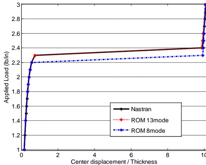
**Figure 7. Clamped-clamped curved beam load-displacement curve of the vertical displacement of the beam center obtained by Nastran and two reduced order models.**
