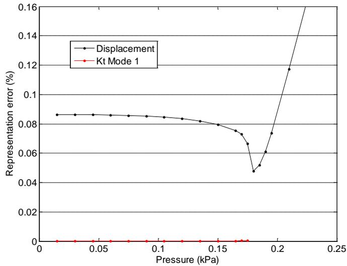
**Figure 16. Representation error  $\varepsilon_{rep}$  of the displacements under downward uniform load on the top wing and of the first eigenvector of the corresponding tangent stiffness matrix, swept wing, 25-mode model.**
